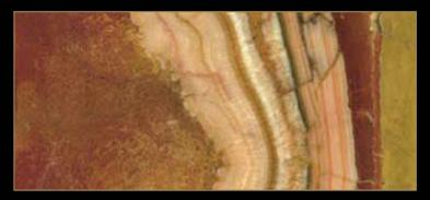
Type: Marble Color: Red Quarry Location: Italy Application: Interior Code: PM / 10062 Bending Strength: 140 - 145 KG/CM<sup>2</sup>
