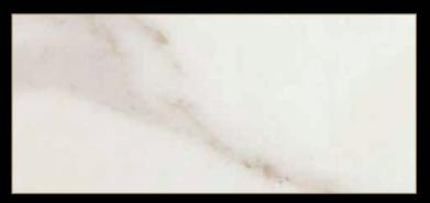
Type: Marble Color: White Quarry Location: Italy Application: Interior - Exterior Code: PM / 10069 Bending Strength: 130 - 180 KG/CM<sup>2</sup>
