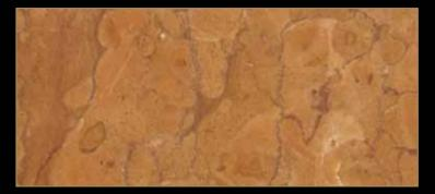
Type: Marble Color: Red Quarry Location: Italy Application: Interior - Exterior Code: PM / 100183 Bending Strength: 95- 105KG/CM<sup>2</sup>
