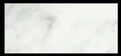
Type: Marble Color: White Quarry Location: Italy Application: Interior - Exterior Code: PM / 10040 Bending Strength: 210 - 222 KG/CM<sup>2</sup>
