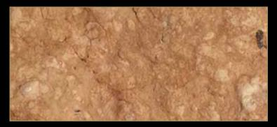
Type: Marble Color: Red Quarry Location: Italy Application: Interior - Exterior Code: PM / 100112 Bending Strength: 148 - 154 KG/CM<sup>2</sup>
