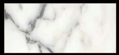
Type: Marble Color: White Quarry Location: Italy Application: Interior - Exterior Code: PM / 100192 Bending Strength: 160 - 180 KG/CM<sup>2</sup>
