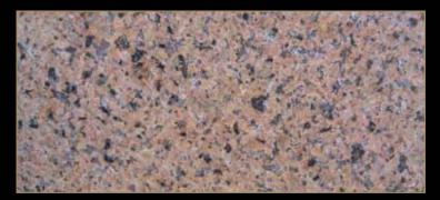
Type: Granite Color: Yellow / Brown Quarry Location: Egypt Application: Interior - Exterior Code: PG / 20025 Bending Strength:2200 - 267 KG/CM<sup>3</sup>
