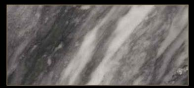
Type: Marble Color: Gray Quarry Location: Italy Application: Interior - Exterior Code: PM / 10036 Bending Strength: 225 - 227 KG/CM<sup>2</sup>
