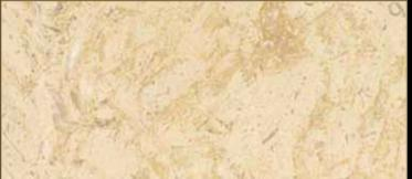
Type: Marble Color: Beige Quarry Location: Italy Application: Interior - Exterior Code: PM / 100150 Bending Strength: 142- 146 KG/CM<sup>2</sup>
