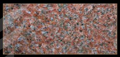
Type: Granite Color: Red Quarry Location: Egypt Application: Interior - Exterior Code: PG / 2002 Bending Strength:2200 - 262 KG/CM<sup>3</sup>
