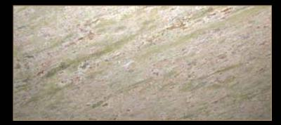
Type: Granite Color: Quarry Location: Brazil Application: Interior - Exterior Code: PG / 200152 Bending Strength: 200- 205 KG/CM<sup>2</sup>
