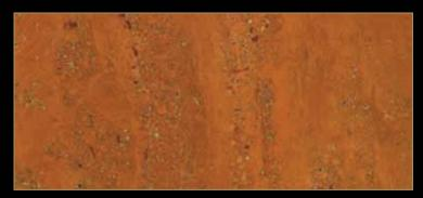
Type: Marble Color: Red Quarry Location: Iran Application: Interior - Exterior Code: PM / 100208 Bending Strength: 110 - 120 KG/CM<sup>2</sup>
