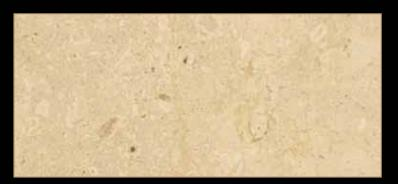
Type: Marble Color: Beige Quarry Location: Italy Application: Interior - Exterior Code: PM / 100198 Bending Strength: 195 - 205 KG/CM<sup>2</sup>
