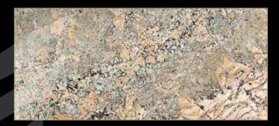
Type: Granite Color: Yellow Quarry Location: Brazil Application: Interior - Exterior Code: PM / 20059 Bending Strength: 175- 180 KG/CM<sup>2</sup>
