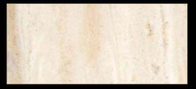
Type: Marble Color: Beige Quarry Location: Italy Application: Interior - Exterior Code: PM / 100143 Bending Strength: 280 - 290 KG/CM<sup>2</sup>
