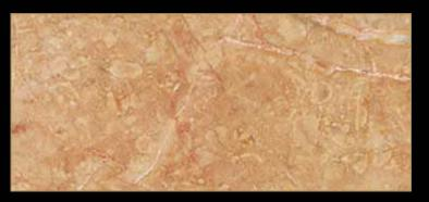
Type: Marble Color: various Quarry Location: Italy Application: Interior Code: PM / 10059 Bending Strength: 110 - 112 KG/CM<sup>2</sup>
