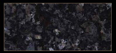
Type: Granite Color: Blue Quarry Location: Norway Application: Interior - Exterior Code: PG / 200101 Bending Strength: 130- 135 KG/CM<sup>2</sup>
