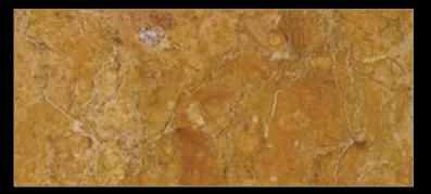
Type: Marble Color: Yellow Quarry Location: Italy Application: Interior - Exterior Code: PM / 10099 Bending Strength: 122 - 128 KG/CM<sup>2</sup>
