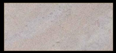
Type: Marble Color: Gray Quarry Location: Italy Application: Interior - Exterior Code: PM / 100144 Bending Strength: 280- 290 KG/CM<sup>2</sup>
