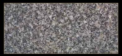
Type: Granite Color: Grey / White Quarry Location: Egypt Application: Interior - Exterior Code: PG/ 20017 Bending Strength:2000 - 262 KG/CM<sup>3</sup>
