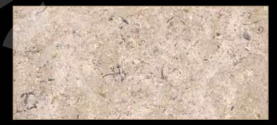
Type: Marble Color: various Quarry Location: Egypt Application: Interior - Exterior Code: PM / 10023 Bending Strength: 180 -185 KG/CM<sup>2</sup>
