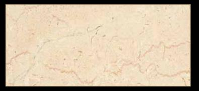
Type: Marble Color: Beige Quarry Location: Italy Application: Interior - Exterior Code: PM / 100199 Bending Strength: 190 - 200 KG/CM<sup>2</sup>
