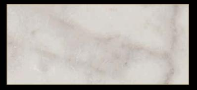
Type: Marble Color: White Quarry Location: Italy Application: Interior - Exterior Code: PM / 10039 Bending Strength: 210 - 222 KG/CM<sup>2</sup>
