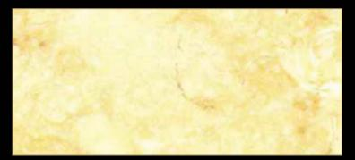
Type: Marble Color: various Quarry Location: Egypt Application: Interior - Exterior Code: PM / 10020 Bending Strength: 170 - 175 KG/CM2
