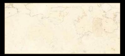
Type: Marble Color: various Quarry Location: Italy Application: Interior - Exterior Code: PM / 10046 Bending Strength: 124 - 128 KG/CM<sup>2</sup>
