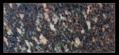
Type: Granite Color: Black Quarry Location: Egypt Application: Interior - Exterior Code: PG / 2007 Bending Strength:4700 - 285 KG/CM<sup>3</sup>
