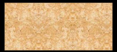
Type: Marble Color: various Quarry Location: Egypt Application: Interior - Exterior Code: PM / 10015 Bending Strength: 170 - 175 KG/CM<sup>2</sup>
