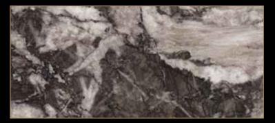
Type: Marble Color: Black Quarry Location: Italy Application: Interior Code: PM / 100103 Bending <u>Strength:</u> 150 - 155 KG/CM<sup>2</sup>
