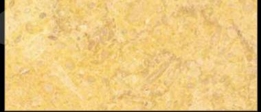
Type: Marble Color: various Quarry Location: Egypt Application: Interior - Exterior Code: PM / 10019 Bending Strength: 196 -198 KG/CM<sup>2</sup>
