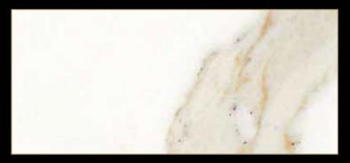
Type: Marble Color: White Quarry Location: Italy Application: Interior - Exterior Code: PM / 10070 Bending Strength: 115 - 155 KG/CM<sup>2</sup>
