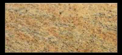
Type: Granite Color: Yellow Quarry Location: Brazil Application: Interior - Exterior Code: PG/ 20095 Bending Strength: 173- 178 KG/CM<sup>2</sup>
