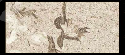
Type: Marble Color: Beige Quarry Location: Italy Application: Interior - Exterior Code: PM / 100162 Bending Strength :195 - 205KG/CM<sup>2</sup>
