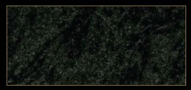
Type: Granite Color: Green Quarry Location: Brazil Application: Interior - Exterior Code: PM / 20041 Bending Strength: 89- 106 KG/CM<sup>2</sup>
