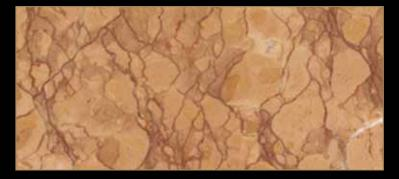
Type: Marble Color: Red Quarry Location: Italy Application: Interior - Exterior Code: PM / 100119 Bending Strength: 148 - 152 KG/CM<sup>2</sup>
