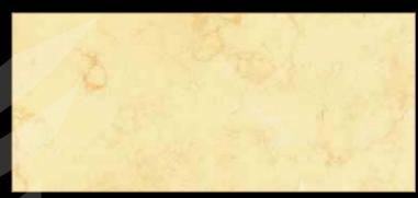
Type: Marble Color: various Quarry Location: Egypt Application: Interior - Exterior Code: PM / 10018 Bending Strength: 145 - 155 KG/CM<sup>2</sup>
