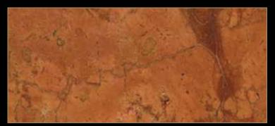
Type: Marble Color: Red Quarry Location: Italy Application: Interior - Exterior Code: PM / 100184 Bending Strength: 95- 105 KG/CM<sup>2</sup>
