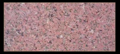
Type: Granite Color: Red Quarry Location: Egypt Application: Interior - Exterior Code: PG/ 20016 Bending Strength:2200 - 263 KG/CM<sup>3</sup>
