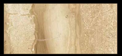
Type: Marble Color: various Quarry Location: Italy Application: Interior Code: PM / 10054 Bending Strength: 152 - 158 KG/CM<sup>2</sup>
