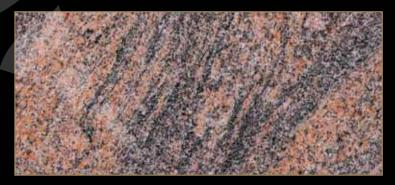
Type: Granite Color: Black Quarry Location: India Application: Interior - Exterior Code: PG / 200115 Bending Strength: 210 - 220 KG/CM<sup>2</sup>
