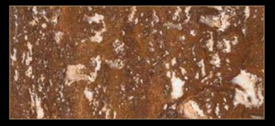
Type: Marble Color: Red Quarry Location: Spain Application: Interior - Exterior Code: PM / 100207 Bending Strength: 145 - 15<u>0 KG/CM<sup>2</sup></u>
