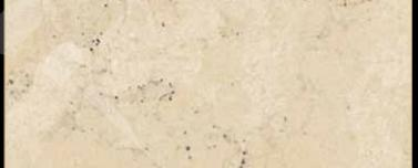
Type: Marble Color: Beige Quarry Location: Italy Application: Interior - Exterior Code: PM / 100114 Bending Strength: 148 - 154 KG/CM<sup>2</sup>
