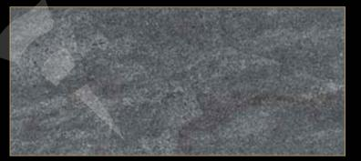
Type: Marble Color: Gray / Blue Quarry Location: Italy Application: Interior - Exterior Code: PM / 100154 Bending Strength: 220 - 225 KG/CM<sup>2</sup>
