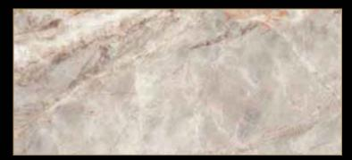
Type: Marble Color: various Quarry Location: Italy Application: Interior Code: PM / 10096 Bending Strength: 17.6 KG/CM<sup>2</sup>
