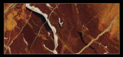
Type: Marble Color: Red Quarry Location: Italy Application: Interior Code: MP / 10084 Bending Strength: 140 - 145 KG/CM<sup>2</sup>
