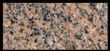
Type: Granite Color: Quarry Location: Italy Application: Interior - Exterior Code: PG / 200150 Bending Strength: 115- 118 KG/CM<sup>2</sup>
