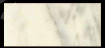
Type: Marble Color: White Quarry Location: U.S.A Application: Interior - Exterior Code: PM / 10026 Bending Strength: 155 - 170 KG/CM<sup>2</sup>
