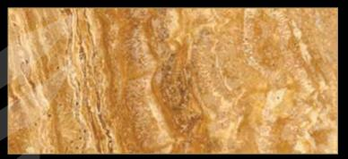
Type: Marble Color: Yellow Quarry Location: Iran Application: Interior - Exterior Code: PM / 100209 Bending Strength: 120 - 130 KG/CM<sup>2</sup>
