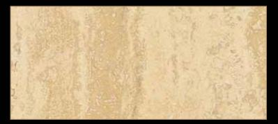
Type: Marble Color: Beige Quarry Location: Italy Application: Interior - Exterior Code: PM / 100200 Bending Strength: 145 - 155 KG/CM<sup>2</sup>
