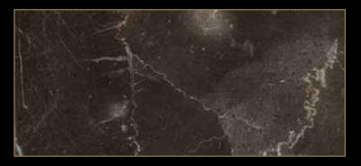
Type: Marble Color: Brown Quarry Location: Spain Application: Interior - Exterior Code: PM / 10094 Bending Strength: 165 - 180 KG/CM<sup>2</sup>
