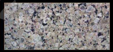
Type: Granite Color: Green Quarry Location: Egypt Application: Interior - Exterior Code: PG / 20027 Bending Strength:2200 - 264 KG/CM<sup>3</sup>
