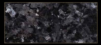
Type: Granite Color: Blue Quarry Location: Norway Application: Interior - Exterior Code: PG/ 200100 Bending Strength: 130- 135 KG/CM<sup>2</sup>
