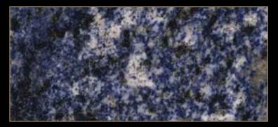
Type: Granite Color: Blue Quarry Location: Brazil Application: Interior - Exterior Code: PG/ 20036 Bending Strength: 165- 175 KG/CM<sup>2</sup>
