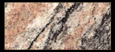
Type: Granite Color: Red Quarry Location: Brazil Application: Interior - Exterior Code: PG/ 20095 Bending Strength: 173- 178 KG/CM<sup>2</sup>
