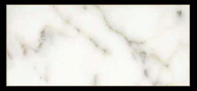
Type: Marble Color: White Quarry Location: Italy Application: Interior - Exterior Code: PM / 100191 Bending Strength: 160 - 180 KG/CM<sup>2</sup>
