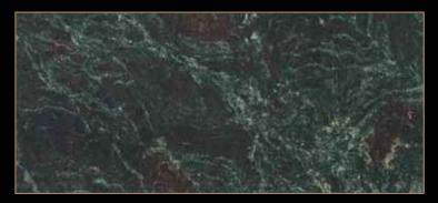
Type: Granite Color: Quarry Location: Brazil Application: Interior - Exterior Code: PG / 200113 Bending Strength: 117 - 124 KG/CM<sup>2</sup>
