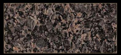
Type: Granite Color: various Quarry Location: Brazil Application: Interior - Exterior Code: PM / 20039 Bending Strength: 180- 185 KG/CM<sup>2</sup>
