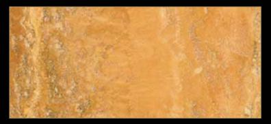
Type: Marble Color: Yellow Quarry Location: Iran Application: Interior - Exterior Code: PM / 100204 Bending Strength: 180 - 190 KG/CM<sup>2</sup>
