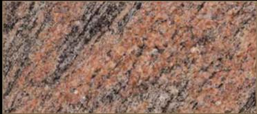
Type: Granite Color: Quarry Location: Brazil Application: Interior - Exterior Code: PG / 200144 Bending Strength: 350- 360 KG/CM<sup>2</sup>
