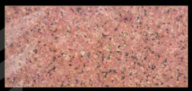
Type: Granite Color: Red Quarry Location: Egypt Application: Interior - Exterior Code: PG / 20018 Bending Strength:1900 - 262 KG/CM<sup>3</sup>
