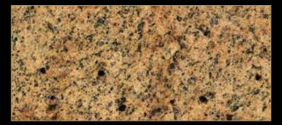
Type: Granite Color: Yellow Quarry Location: India Application: Interior - Exterior Code: PG / 200112 Bending Strength: 117 -124 KG/CM<sup>2</sup>
