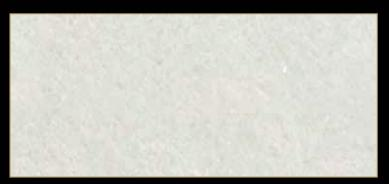
Type: Marble Color: White Quarry Location: Greece Application: Interior - Exterior Code: PM / 100142 Bending Strength: 100 - 110 KG/CM<sup>2</sup>
