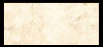
Type: Marble Color: White Quarry Location: Greece Application: Interior - Exterior Code: PM / 100214 Bending Strength: 136 - 165 KG/CM<sup>2</sup>
