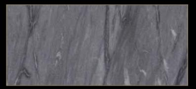
Type: Marble Color: Dark Gray Quarry Location: Italy Application: Interior - Exterior Code: PM / 10035 Bending Strength: 220 - 233 KG/CM<sup>2</sup>
