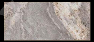
Type: Marble Color: Gray Quarry Location: Italy Application: Interior - Exterior Code: PM / 100146 Bending Strength: 280- 290KG/CM<sup>2</sup>
