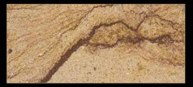
Type: Marble Color: Beige Quarry Location: Italy Application: Interior - Exterior Code: PM / 100155 Bending Strength: 69 - 72 KG/CM<sup>2</sup>
