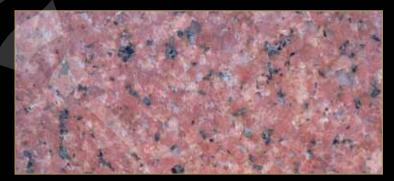
Type: Granite Color: Red Quarry Location: Egypt Application: Interior - Exterior Code: PG / 20019 Bending Strength: 1900 - 262 KG/CM<sup>3</sup>
