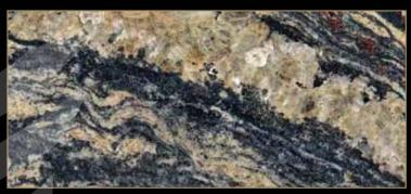
Type: Granite Color: Quarry Location: Brazil Application: Interior - Exterior Code: PG / 200114 Bending Strength: 80 - 93 KG/CM<sup>2</sup>
