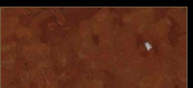
Type: Marble Color: Red Quarry Location: Italy Application: Interior Code: PM / 100180 Bending Strength: 106 - 108 KG/CM<sup>2</sup>
