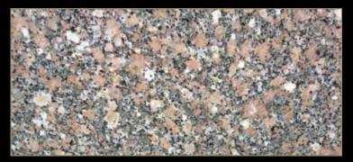
Type: Granite Color: Red Quarry Location: Egypt Application: Interior - Exterior Code: PG / 2004 Bending Strength:2400 - 264 KG/CM<sup>3</sup>
