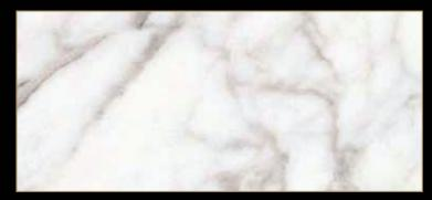
Type: Marble Color: White Quarry Location: Italy Application: Interior - Exterior Code: PM / 10044 Bending Strength: 205 - 220 KG/CM<sup>2</sup>
