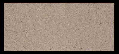
Type: Marble Color: various Quarry Location: Italy Application: Interior - Exterior Code: PM / 100156 Bending Strength: 56 - 58 KG/CM<sup>2</sup>
