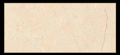
Type: Marble Color: Beige Quarry Location: Italy Application: Interior Code: PM / 100104 Bending Strength: 180 - 185 KG/CM<sup>2</sup>
