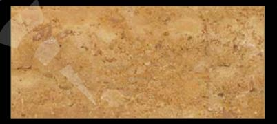
Type: Marble Color: Yellow Quarry Location: Italy Application: Interior - Exterior Code: PM / 100210 Bending Strength: ------
