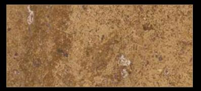
Type: Marble Color: Beige Quarry Location: Italy Application: Interior - Exterior Code: PM / 100203 Bending Strength: 140 - 150 KG/CM<sup>2</sup>
