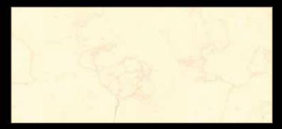
Type: Marble Color: White Quarry Location: Egypt Application: Interior - Exterior Code: PM / 10021 Bending Strength: 145 - 155 KG/CM<sup>2</sup>
