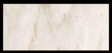
Type: Marble Color: White Quarry Location: Italy Application: Interior - Exterior Code: PM / 100190 Bending Strength: 165 - 175 KG/CM<sup>2</sup>
