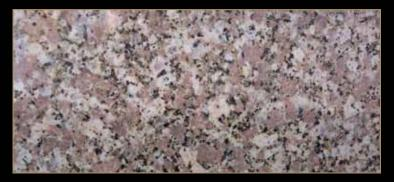
Type: Granite Color: various Quarry Location: Egypt Application: Interior - Exterior Code: PG/ 20020 Bending Strength:2200 - 261 KG/CM<sup>3</sup>
