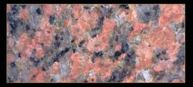
Type: Granite Color: Red Quarry Location: Egypt Application: Interior - Exterior Code: PG / 20012 Bending Strength:2200 - 267 KG/CM<sup>3</sup>
