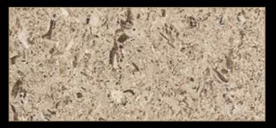
Type: Marble Color: various Quarry Location: Italy Application: Interior - Exterior Code: PM / 10095 Bending Strength: 140 - 150 KG/CM<sup>2</sup>
