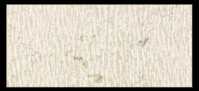
Type: Marble Color: Beige Quarry Location: Italy Application: Interior - Exterior Code: PM / 100116 Bending Strength: 148 - 154 KG/CM<sup>2</sup>
