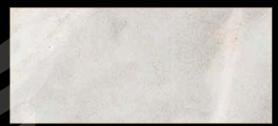
Type: Marble Color: White Quarry Location: Italy Application: Interior - Exterior Code: PM / 100145 Bending Strength: 280- 290 KG/CM<sup>2</sup>
