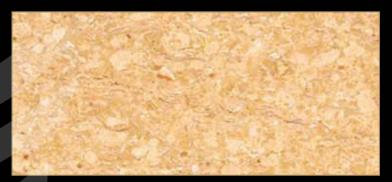
Type: Marble Color: Yellow Quarry Location: Spain Application: Interior - Exterior Code: PM / 10097 Bending Strength: 16.5 KG/CM<sup>2</sup>
