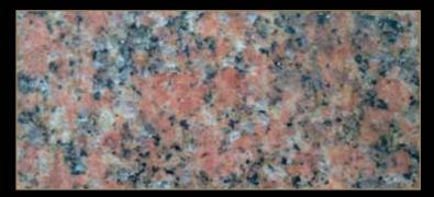
Type: Granite Color: Red Quarry Location: Egypt Application: Interior - Exterior Code: PG/ 20023 Bending Strength:2200 - 263 KG/CM<sup>3</sup>
