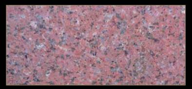
Type: Granite Color: Red Quarry Location: Egypt Application: Interior - Exterior Code: PG / 20015 Bending Strength:2200 - 267 KG/CM<sup>3</sup>
