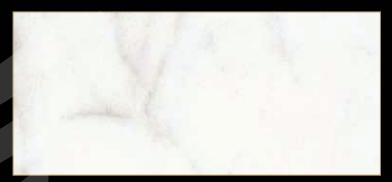
Type: Marble Color: White Quarry Location: Italy Application: Interior - Exterior Code: PM / 10041 Bending Strength: 210 - 222 KG/CM<sup>2</sup>
