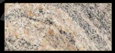
Type: Granite Color: Quarry Location: Brazil Application: Interior - Exterior Code: PG / 20099 Bending Strength: 125- 130 KG/CM<sup>2</sup>
