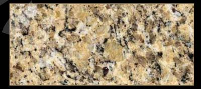
Type: Granite Color: Yellow Quarry Location: Brazil Application: Interior - Exterior Code: PM / 20060 Bending Strength: 143 - 152 KG/CM<sup>2</sup>
