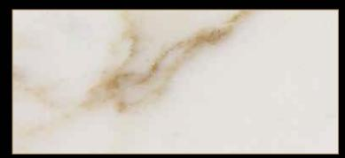
Type: Marble Color: White Quarry Location: Italy Application: Interior - Exterior Code: PM / 10072 Bending Strength: 130 - 180 KG/CM<sup>2</sup>
