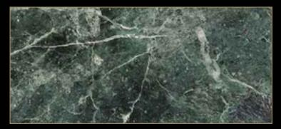
Type: Marble Color: Green Quarry Location: Italy Application Interior - Exterior Code: PM / 100224 Bending Strength: 220 - 230 KG/CM<sup>2</sup>
