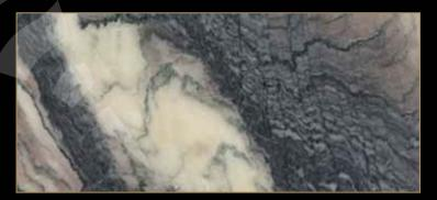
Type: Marble Color: various Quarry Location: Italy Application: Interior - Exterior Code: PM / 100122 Bending Strength: 90 - 100 KG/CM<sup>2</sup>
