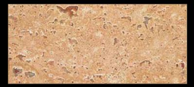
Type: Marble Color: Red Quarry Location: Iran Application: Interior - Exterior Code: 10086 Bending Strength: 118 - 122 KG/CM<sup>2</sup>
