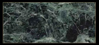
Type: Marble Color: Green Quarry Location: Italy Application: Interior - Exterior Code: PM / 100215 Bending Strength: 220 - 230 KG/CM<sup>2</sup>
