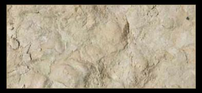
Type: Marble Color: Beige Quarry Location: Italy Application: Interior - Exterior Code: PM / 100115 Bending Strength: 148 - 154 KG/CM<sup>2</sup>
