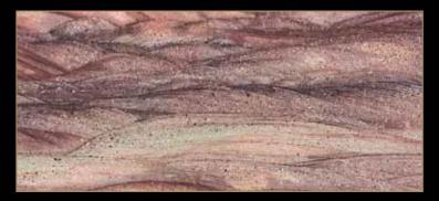
Type: Granite Color: Various Quarry Location: Brazil Application: Interior - Exterior Code: PM / 20051 Bending Strength: 168 KG/CM<sup>2</sup>
