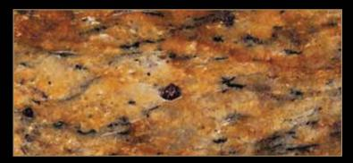
Type: Granite Color: Yellow Quarry Location: Brazil Application: Interior - Exterior Code: PM / 20092 Bending Strength: 65- 75 KG/CM2
