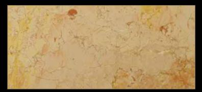
Type: Marble Color: various Quarry Location: Egypt Application: Interior - Exterior Code: PM / 10016 Bending Strength: 170 - 175 KG/CM<sup>2</sup>
