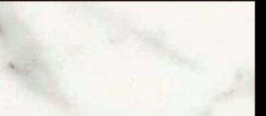
Type: Marble Color: White Quarry Location: Italy Application: Interior - Exterior Code: PM / 100189 Bending Strength: 165 - 175 KG/CM<sup>2</sup>
