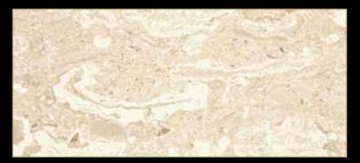
Type: Marble Color: Beige Quarry Location: Italy Application: Interior - Exterior Code: PM / 100148 Bending Strength: 128- 132 KG/CM<sup>2</sup>
