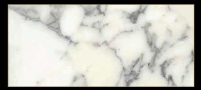
Type: Marble Color: Gray Quarry Location: Italy Application: Interior - Exterior Code: PM / 10028 Bending Strength: 160 - 180 KG/CM<sup>2</sup>
