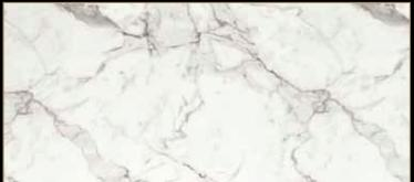
Type: Marble Color: White Quarry Location: Italy Application: Interior - Exterior Code: PM / 10067 Bending Strength: 130 - 180 KG/CM<sup>2</sup>
