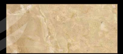
Type: Marble Color: various Quarry Location: Italy Application: Interior Code: PM / 10057 Bending Strength: 125 - 130 KG/CM<sup>2</sup>
