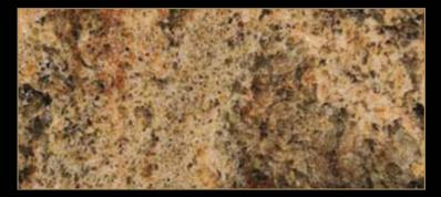
Type: Granite Color: Red Quarry Location: Brazil Application: Interior - Exterior Code: PM / 20047 Bending Strength: 100- 110 KG/CM<sup>2</sup>
