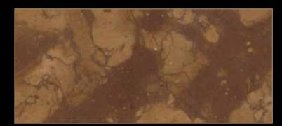
Type: Marble Color: Red Quarry Location: Italy Application: Interior - Exterior Code: PM / 100182 Bending Strength: 155 - 160 KG/CM2
