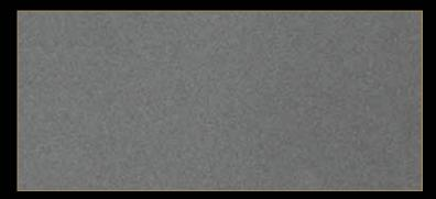
Type: Granite Color: White / Grey Quarry Location: Brazil Application: Interior - Exterior Code: PG / 200144 Bending Strength: 350- 360 KG/CM<sup>2</sup>
