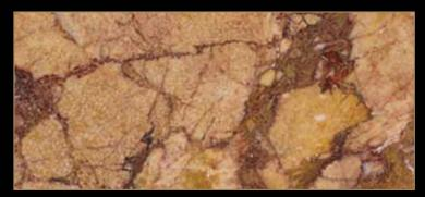
Type: Marble Color: various Quarry Location: Italy Application: Interior Code: PM / 10060 Bending Strength: 110 - 115 KG/CM<sup>2</sup>
