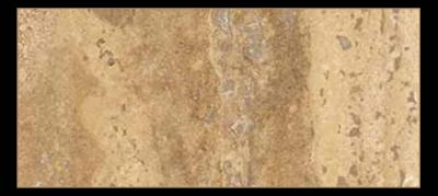
Type: Marble Color: Beige Quarry Location: Italy Application: Interior - Exterior Code: PM / 100206 Bending Strength: 135 - 145 KG/CM<sup>2</sup>
