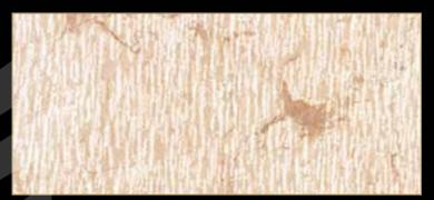
Type: Marble Color: Red Quarry Location: Italy Application: Interior - Exterior Code: PM / 100113 Bending Strength: 148 - 154 KG/CM<sup>2</sup>
