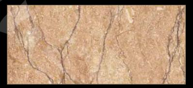
Type: Marble Color: Red Quarry Location: Italy Application: Interior - Exterior Code: PM / 10074 Bending Strength : 170 - 180 KG/CM<sup>2</sup>
