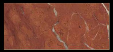
Type: Marble Color: Red Quarry Location: Spain Application: Interior - Exterior Code: PM / 100172 Bending Strength: 85 - 93 KG/CM<sup>2</sup>
