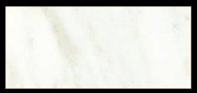
Type: Marble Color: White Quarry Location: Greece Application: Interior - Exterior Code: PM / 10085 Bending Strength: 196 KG/CM<sup>2</sup>
