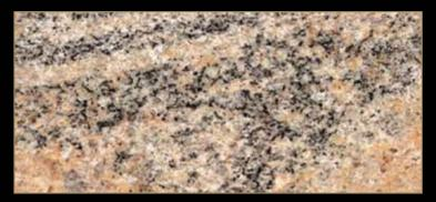
Type: Granite Color: Various Quarry Location: India Application: Interior - Exterior Code: PM / 20079 Bending Strength: 94- 98 KG/CM<sup>2</sup>
