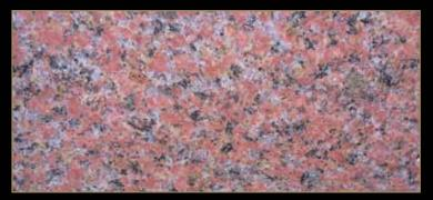
Type: Granite Color: Red Quarry Location: Egypt Application: Interior - Exterior Code: PG / 2008 Bending Strength:2200 - 262 KG/CM<sup>3</sup>
