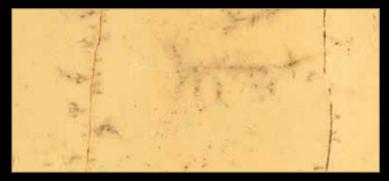
Type: Marble Color: Yellow Quarry Location: Spain Application: Interior - Exterior Code: PM / 100102 Bending Strength: 105 - 110 KG/CM<sup>2</sup>
