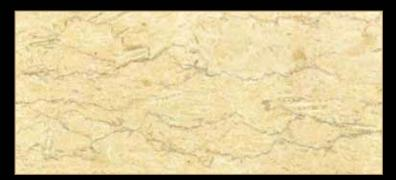
Type: Marble Color: various Quarry Location: Egypt Application: Interior - Exterior Code: PM / 10017 Bending Strength: 180 -185 KG/CM<sup>2</sup>
